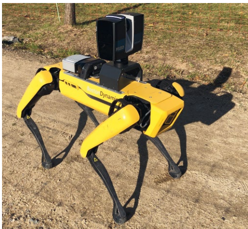
Bild 29 Roboter Boston Dynamics Spot mit Edge-Computer, Adapter und Faro Focus Laserscanner Robot Boston Dynamics Spot with edge-computer, adapter and Faro Focus Laserscanner
