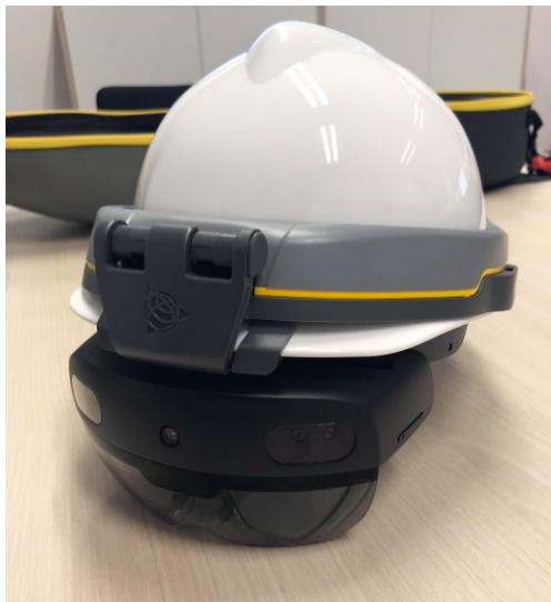
Bild 25 Microsoft HoloLens 2 am Bauhelm Trimble XR10 Microsoft HoloLens 2 integrated into helmet Trimble XR10
